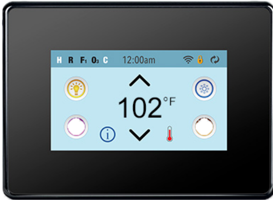
Figure 1: SpaTouch2 touchscreen control panel
