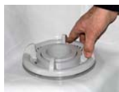
Turn filter housing ring counter-clockwise to remove housing and telescoping weir.
